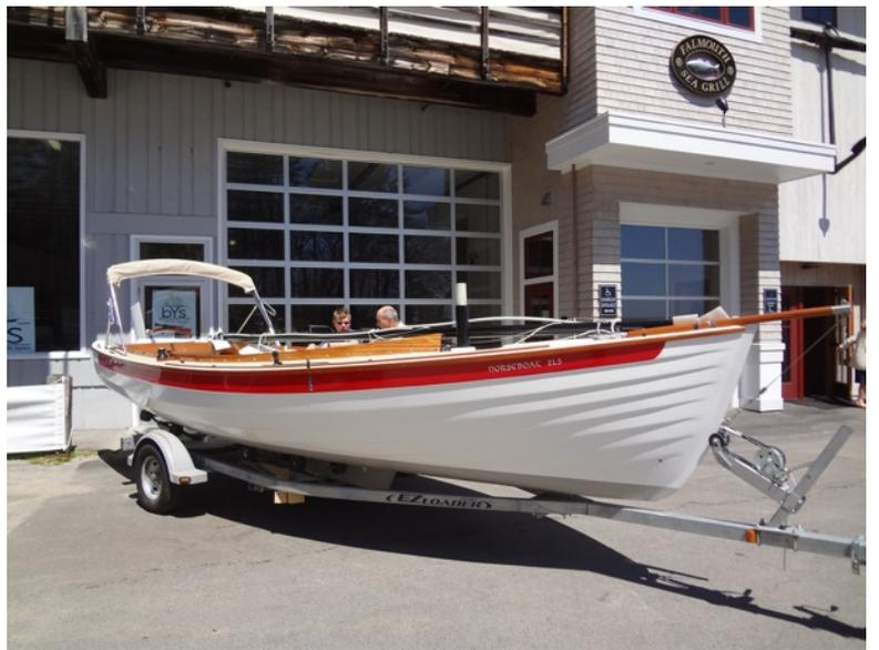
The 21.5 Cabin and Open models have the same innovative fiberglass hull. The Cabin model has a fiberglass interior and deck. The Open model has a wood/epoxy composite deck with varnished wood coaming, similar to the NorseBoat 12.5 and 17.5 models.
