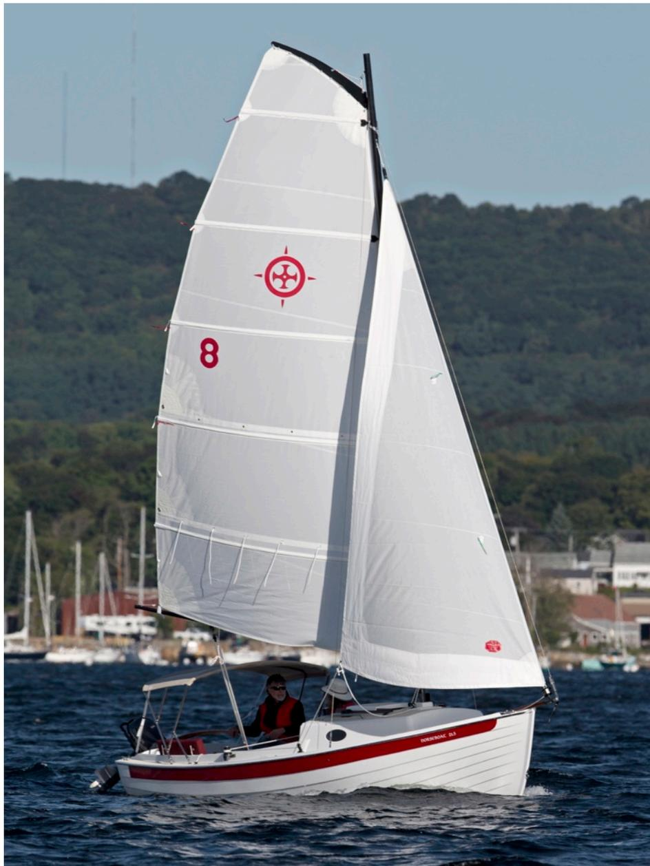
The NorseBoat 21.5 is relatively lightweight, with a sailing displacement-to-length ratio of 150. A ballasted foil-shaped stub keel, modest-size pivoting centerboard and kick-up rudder provide good stability with shallow draft. The spacious cockpit seats eight and has large storage lockers for gear.
