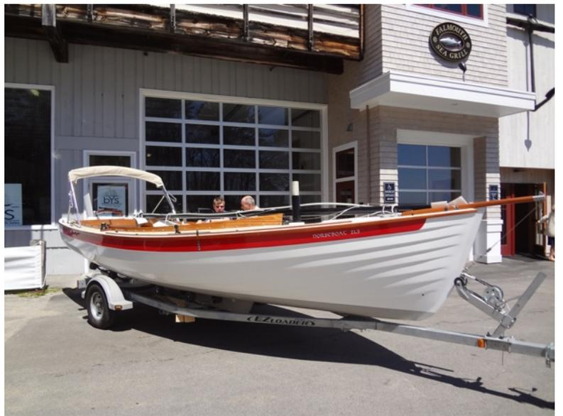
The 21.5 Cabin and Open models have the same innovative fiberglass hull. The balance of the build for both models is a high-quality wood/epoxy/glass composite. The Open model has a varnished wood coaming, similar to the NorseBoat 12.5 and 17.5 models.
